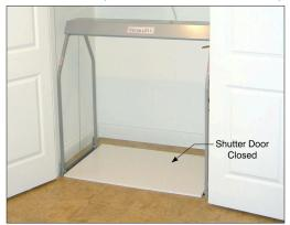
The Auto-Shutter automatically deploys a shutter door to cover the Versa Lift opening whenever the lifting platform is lowered. This accessory is required whenever the Versa Lift is installed inside the living space of a home, or in a closet, or in an attic space accessible by a passage door from a living space, or on a deck, or any other area where children or pets might have ready access to the lift opening.
