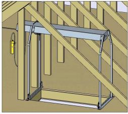
The Truss Leg Kit adapts the Versa Lift 24 to fit between roof trusses on 24" centers. Usually the Versa Lift will not fit between roof truss members on 24" centers. (Roof trusses must not be cut or modified because each member is load bearing within the assembly.)
