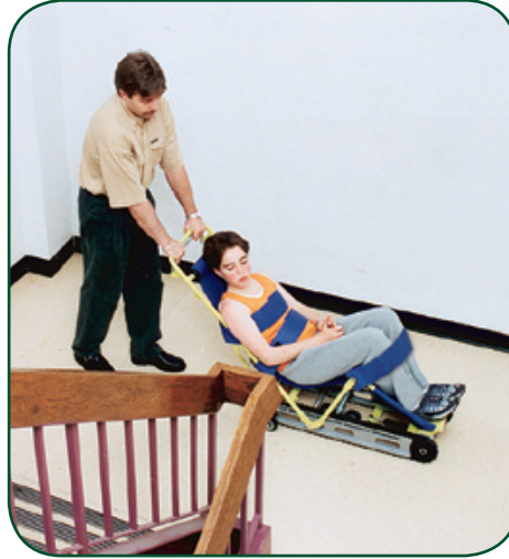
To turn the Evacu-Trac on flat surfaces, the attendant pushes down on the handle and pivots the unit on the rear auxiliary wheels.
